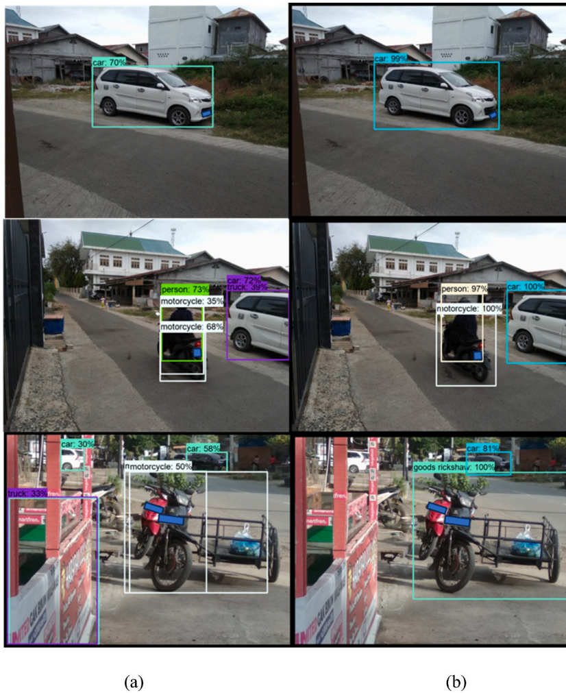
Fig. 11. Experimental object classification under evening illumination. (a) before training. (b) after training.
