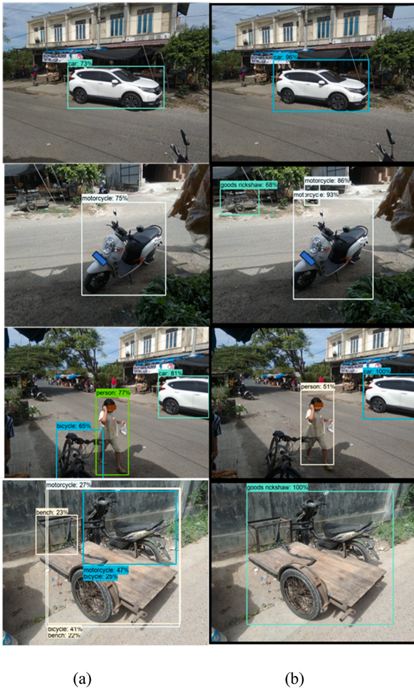
Fig. 9. Experimental object classification under morning illumination. (a) before training. (b) after training.
