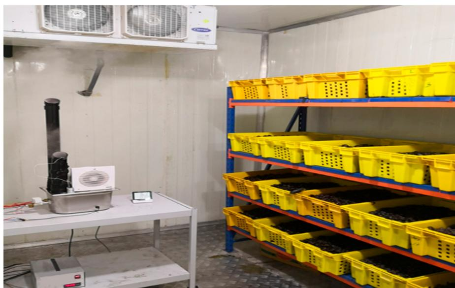
**Figure 5.** The experimental setup in the controlled cold storage room showing the designed humidifier and crates of stored dates.
