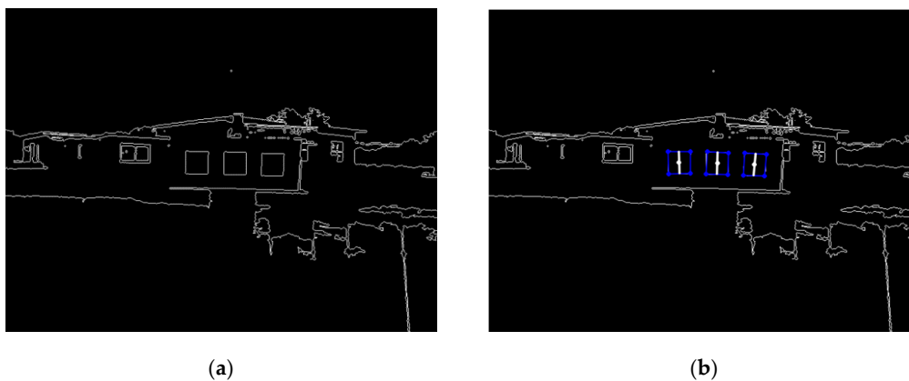
Figure 3. Image processing for marker detection. (a) Contour image; (b) Detected marker.
