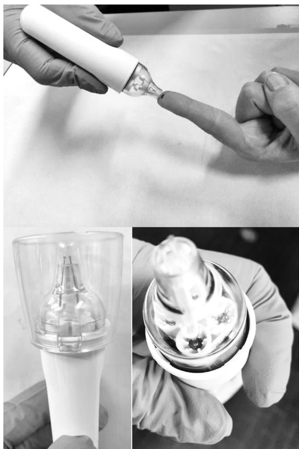
Fig. 3. (a) Capillary DBS sampling from a fingerprick, (b) in-device filled capillaries before generating DBS and (c) the obtained fixed-volume, pre-cut DBS within the device.
