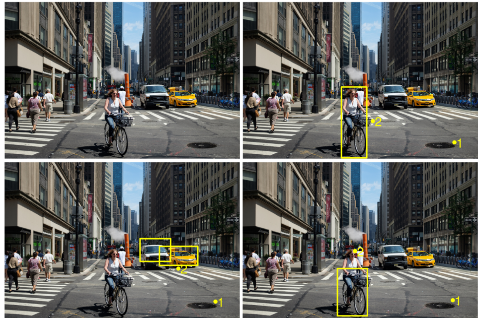
Fig 8. Fixation locations and bounding box predictions of the FOD for three different object classes (person, car and bicycle) but for the same image and initial point of fixation. Top-left: original image (source: https://www.flickr.com/photos/kristoffer-trolle/27882648666/ with Creative Commons license.), top-right: person detection, bottom-left: car detections, bottom-right: bicycle detection. Yellow dots show fixation points, numbers in yellow fonts indicate the sequence of fixations and the bounding boxes are the final detections.
