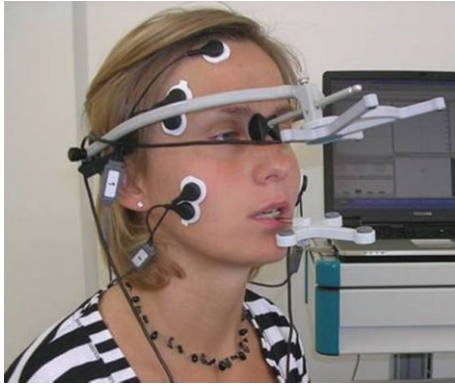
FIGURE 2: Jaw Motion Analysis system mounted on subject. Courtesy of Zebbris Medical GmbH.
