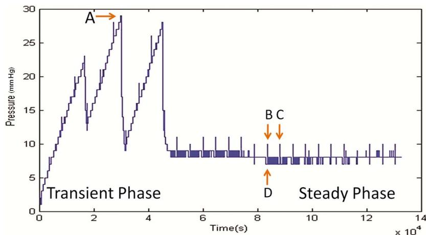
**Figure 4.** Pressure versus time curve during flow characterization of AGV number 1. A Peak pressure in the transient phase, B and C opening pressure, and D closing pressure.
