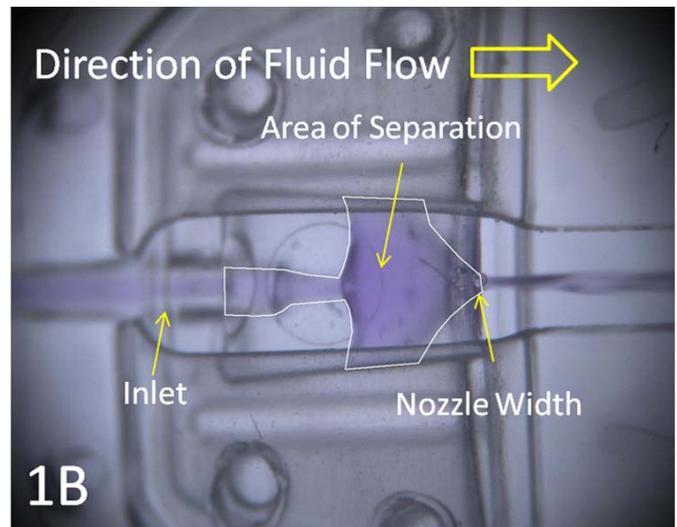
**Figure 1.** (A) Experimental setup of priming, (B) Area of separation of valve leaflets and nozzle width during priming.
