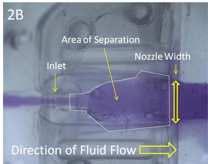
**Figure 2.** (A) Experimental setup of flow characterization, (B) Area of separation of valve leaflets and nozzle width subsequent to flow characterization.
