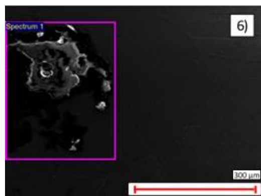
Figure 13. SEM image of contamination on the SS with Ni coating thin-walled pipe (62.7% C, 35.1% Ni, 0.99% Fe, 0.86% O, 0.20% Cr, and 0.13% Al) (6).
