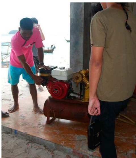
Figure 1. Compressed air machine for generating plain air to the diver during fishing dive.
