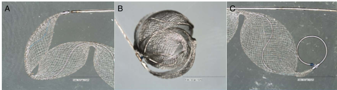
Figure 1 The Medina Embolic Device (MED) seen straightened out (A and C) and in its spherical form (B).
