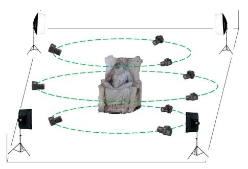
Figure 4. Layout of the photogrammetric acquisition area.
