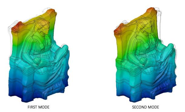
**Figure 11.** Modal analysis of *Mater Matuta*: first (left— $f_1$  = 122.2 Hz) and second (left— $f_2$  = 183.6 Hz) mode; displacement mapping color code ranges between blue (still points) to red (maximum modal displacements).
