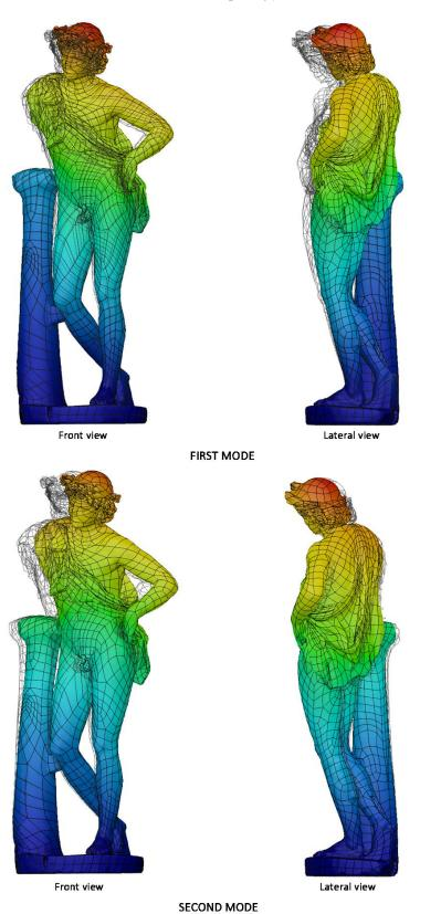
homogeneous 3D FE model of the asset. Two viewpoints are reported for each modal shape, associated with the first modal frequency  $f_1$  =20.7 Hz and the second one  $f_2$  = 46.5 Hz.
