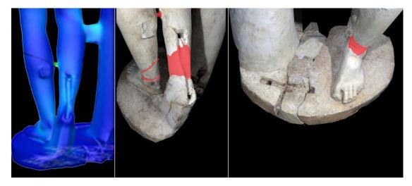
Figure 23. Results of static stress analysis versus previous restoration works.
