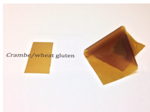
Figure 2: Compression-molded films. Extruded material compression-molded, without a frame, into thin, translucent films using a 130 °C press temperature at 75 bar for 10 min. The flat and wrinkled films are from the same material. The width of the left film is ~17 mm. Please click here to view a larger version of this figure.
