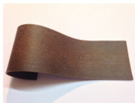
Figure 1: Extruded material. Extruded film using a die temperature of 130 °C. It contains 35.7 wt% crambe, 23.8 wt% wheat gluten, 25.5 wt% glycerol, and 15 wt% urea. The width of the film is 44 mm. Please click here to view a larger version of this figure.
