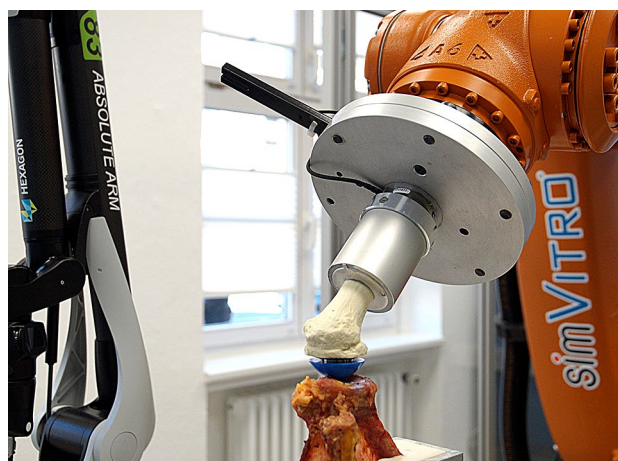
Fig. 1 Human specimen in robotic test setup; experimental setup consisting of 3D measuring arm, industrial robot, force torque sensor, artificial bone with stemless shoulder implant and human cadaveric scapula. The humeral head is shifted in the 3 o'clock direction to perform an anterior dislocation
