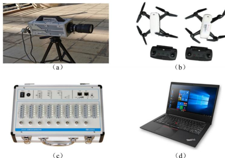
**Figure 5.** Experimental equipment: (a) Fixed camera; (b) DJI drone; (c) JMTEST acquisition instrument; (d) JMTEST dynamic acquisition software.
