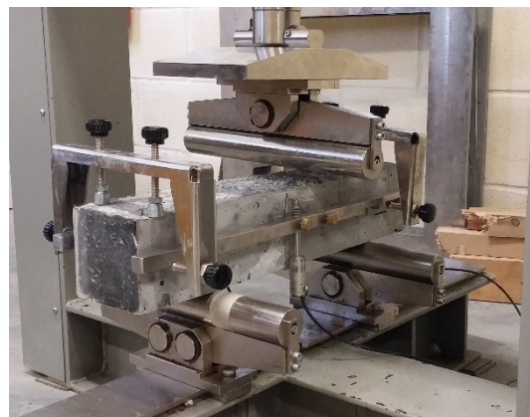
Figure 5. Set-up of flexural tension test.
