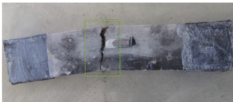
Figure 14. Failure of beam (direct tension test) from mixture 2(0-2)/16/6.1.
