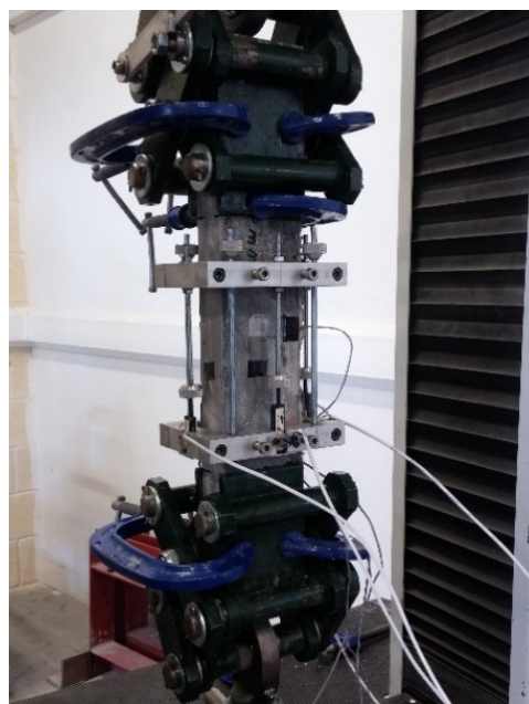
Figure 3. Set-up of direct tension test.
