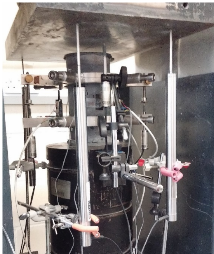
Figure 1. Set-up of uniaxial compression test.
