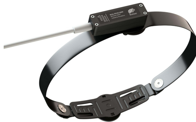
Figure 1 Headband used on patients' heads for the Brain4care non-invasive ICP measuring device.
