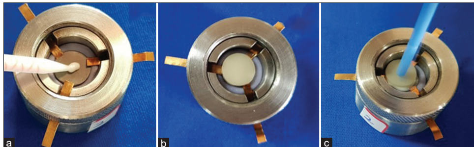
Figure 10: (a) Dispensing of resin cement. (b) Placement of ceramic disc. (c) Pressure applied to remove excess cement
