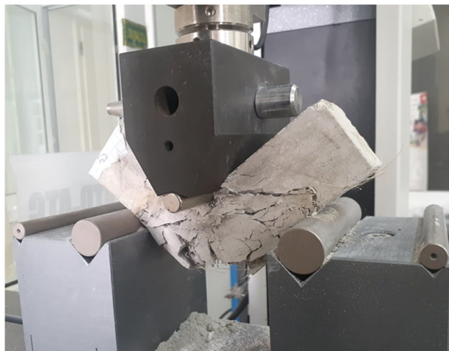
Figure 12. Flexural strength test of (M4L6) concrete reinforced with horizontal AAF fibers.
