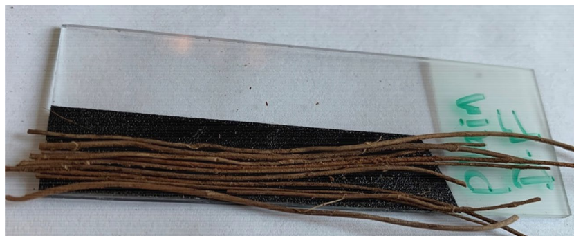
Figure 2. Fiber arrangement on a glass slide for contact angle measurement.
