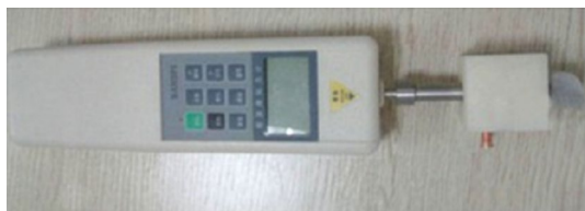
Fig. 7 Abdominal wall tensiometer. Tensiometer used by Chen et al. to measure the required thrust (N) to produce displacement (mm) (adapted with permission from Chen et al. [22])
