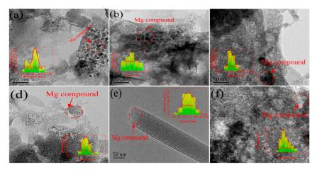
**Figure 1.** HRTEM images of six different Mg-loaded biochars. (**a**; **b**; **c**; **d**; **e**; and **f** represent BSB, FSB, MSB, CFSB, TSB, and CSB, respectively).
