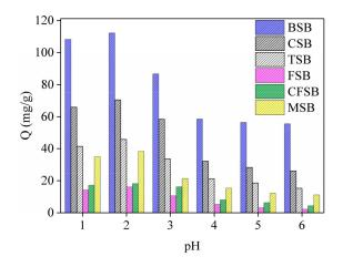
Figure 5. Effect of adsorption on Cr(VI) at different pH values.
