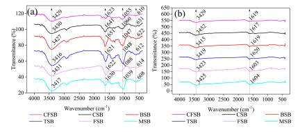
Figure 2. FTIR spectra of the six different biochars (a) before and (b) after adsorption of Cr(VI).
