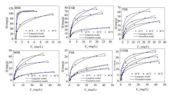
Figure 7. Adsorption isotherms of Cr(VI) for six different biochars.
