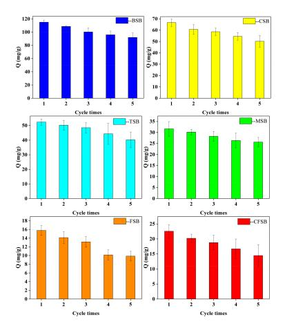
Figure 8. Recycle adsorption performance in wastewater of Cr(VI) adsorption by Mg-loaded biochars.
