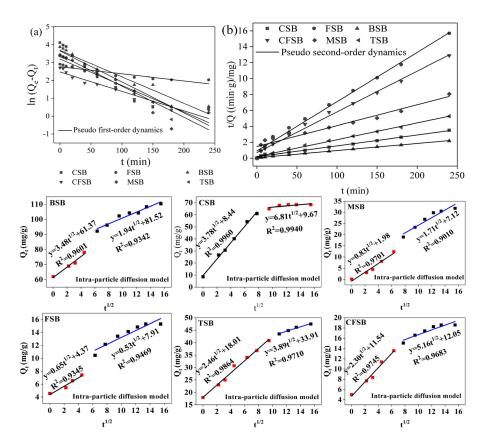
**Figure 6.** Adsorption kinetic curves of Cr(VI) on the six biochars ((**a**): Pseudo first-order dynamics fitting curve; (**b**): Pseudo second-order dynamics fitting curve).
