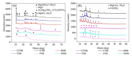
Figure 4. XRD analysis of the six biochars (a) before and (b) after adsorption of Cr(VI).
