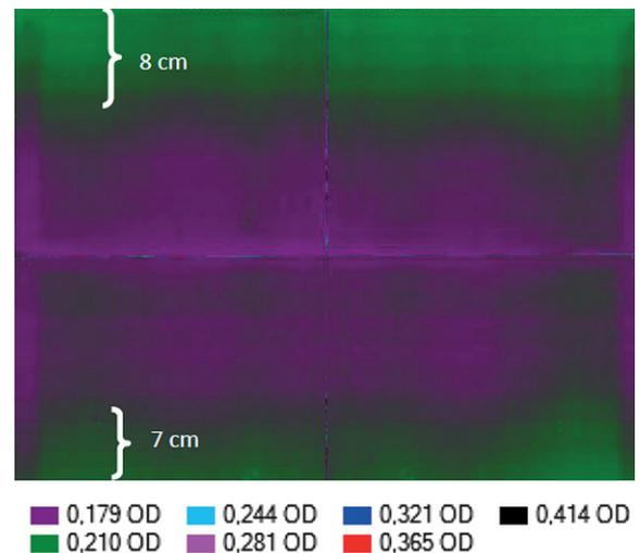
FIGURE 1. Inhomogeneity map of the full scanning surface (A) and the homogeneous area in the centre of the scanner glass (B).
