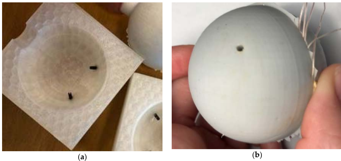
Figure 3. 3D printed mold and resulting rubber sphere molded concentrically over a steel sphere: (a) 3D printed rubber mold; (b) Demolded rubber assembly.
