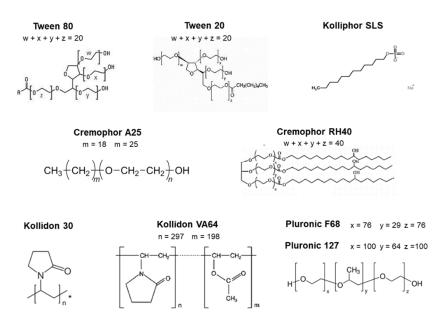
**Figure A1.** Chemical structures of the investigated surfactants and solubilizers. \* Kollidon 30 is a medium molecular povidone with a molecular weight of 44,000–54,000 g/mol.
