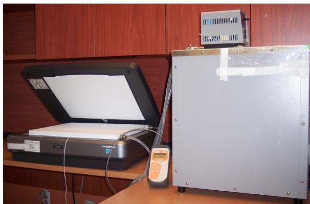
FIG. 1. Scanner bed temperature experimental setup: water coming from the heating/refrigerating pump to the right is circulated inside a hollow slab placed over the reflector, which is over the scanner bed and the film. A small surface thermistor is placed at the slab–reflector interface.
