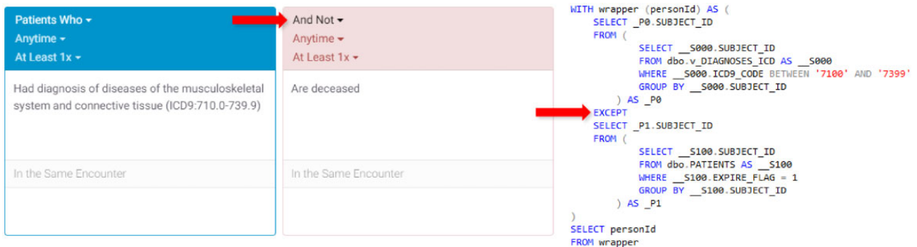
Figure 5. Visual representation of a 2-panel query with the user interface on the left and corresponding compiled SQL representation on the right. The second panel is used as an exclusion criteria and executed using a SQL EXCEPT statement.
