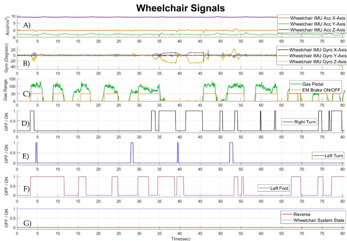
Figure 13. Signals from the wheelchair head-foot steering system of a DCP patient, while he was performing standardized wheelchair start and stop driving task. (A) Signals from the accelerometer of the IMU mounted on the wheelchair. (B) Signals from the gyroscope of the IMU mounted on the wheelchair. (C) Signal from the gas pedal of the wheelchair (green color); and signal from the EM brake of the wheelchair (orange color). (D) Signal from the sensor of the wheelchair responsible for right steering (E) Signal from the sensor of the wheelchair responsible for left steering (F) Signal from the sensor mounted on the left foot support of the wheelchair (G) Signal that shows if reverse wheelchair movement is enabled (red color); and signal that shows whether the wheelchair is enabled (blue color).
