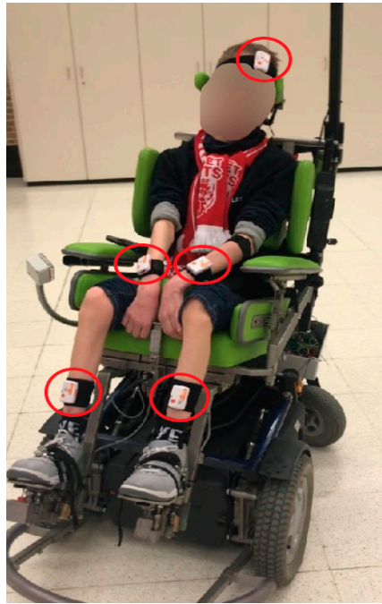
Figure 6. The five IMUs placed on a DCP patient while driving the head-foot wheelchair steering system. The IMUs are positioned on the right and left distal arm, on the right and left tibialis anterior, and on the forehead, respectively.
