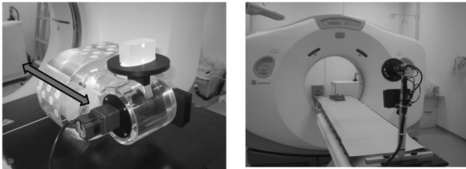
FIG. 2. The respiratory motion phantom has sinusoidal movements. Target displacement occurs in the cranial–caudal direction (bidirectional arrow) with variable velocity and amplitude.
