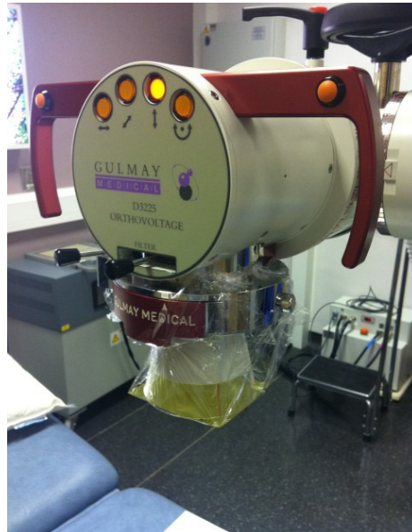
FIG. 2. Film piece positioned with cling film at the end of the applicator, simulating conditions of no backscatter.
