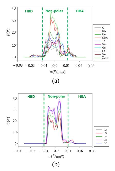
**Figure 3.** σ-profiles of (**a**) DES components and (**b**) siloxanes.
