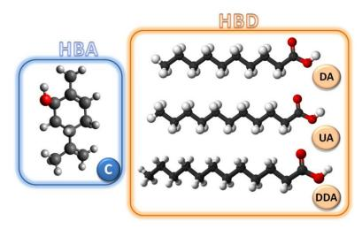
Figure 18. Structures of HBA and HBD used for DES synthesis.
