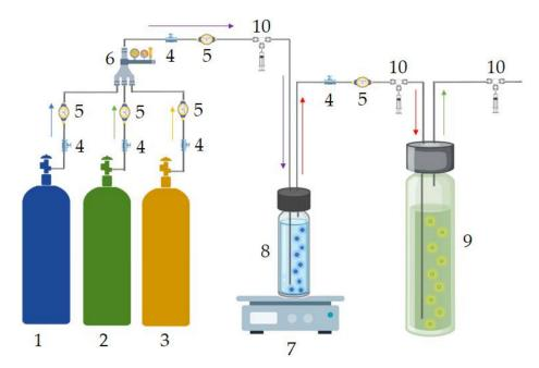
**Figure 19.** Siloxane absorption installation: 1-N<sub>2</sub> bottle; 2-CH<sub>4</sub> bottle; 3-CO<sub>2</sub> bottle; 4-valve; 5-flowmeter; 6-gas mixer; 7-hotplate; 8-vial with siloxanes; 9-vial with DES; 10-gas sample collection point.
