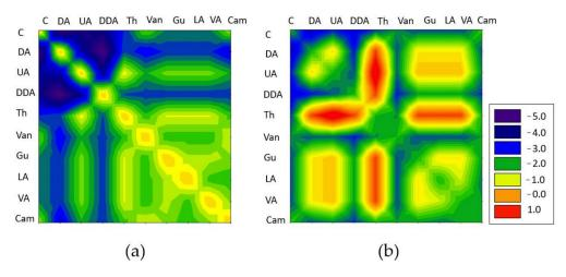
**Figure 2.** Screening of logarithmic activity coefficients of (a) L2 and (b) D3 in various DES mixtures at a 1:1 molar ratio.
