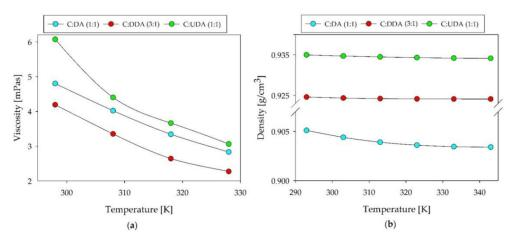
Figure 8. (a) Viscosity and (b) density of the new DESs.
