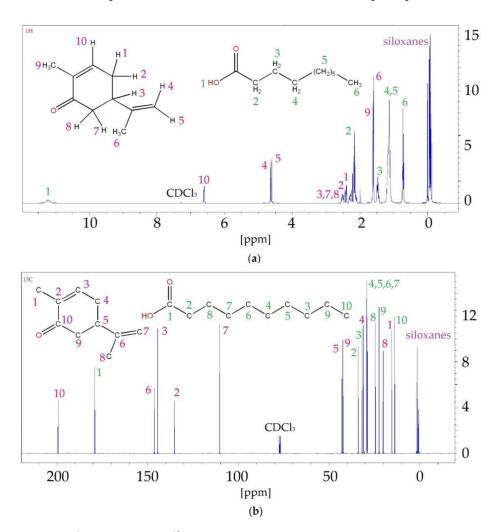
**Figure 14.** <sup>1</sup>H NMR (**a**) and <sup>13</sup>C NMR (**b**) spectra for C:DA (1:1) after the absorption process of siloxanes from the model biogas stream.
