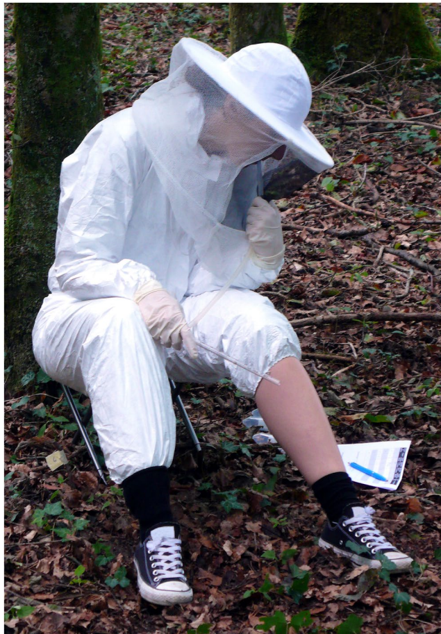
Figure 1. The human landing catch (HLC) method for measuring the efficacy of topical repellents under field conditions. Mosquitoes alighting on the treated and exposed lower leg were aspirated by a mouth aspirator and kept in Falcon tubes for species identification in the laboratory. Apart from the treated area the whole body was fully protected by a jump suit, a bee keeper's hat and latex gloves through which mosquitoes cannot bite.
