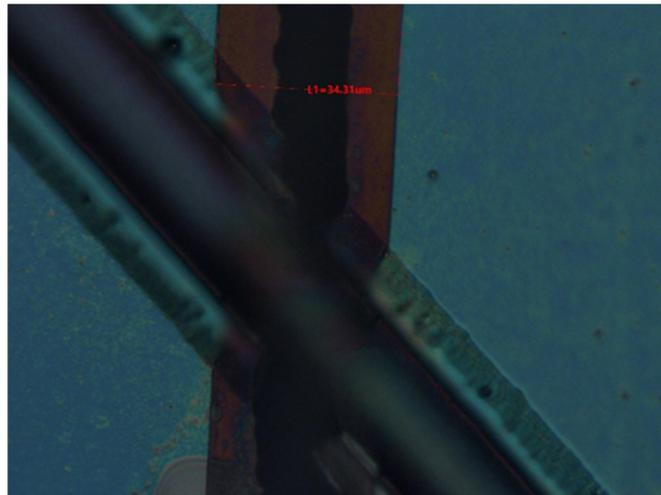
**Figure 9.** The width of bottom channel measured by metallographic microscope.
