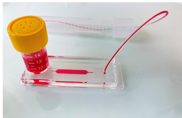
Fig. 3. 3D Spheroid PDMS chip. PDMS microsystem for spheroid cell culture in a 60 \times 22 mm slide. Microsystem is constituted by a reservoir for media (a 15 ml Falcon tube cut at desired size) glued to the PDMS microsystem. The reservoir is connected to the cell culture chamber by an 8 mm length channel (200 \mu\text{m} wide and 70 \mu\text{m} high). Cell culture chamber is 4 mm wide by 20 mm long (height 200 \mu\text{m} ). To slowdown media flow, a 2 cm long serpentine channel (200 \mu\text{m} wide 70 \mu\text{m} high) was placed after the cell chamber. Output through 1.5 mm Tygon tubing with 500 \mu\text{m} internal diameter.
