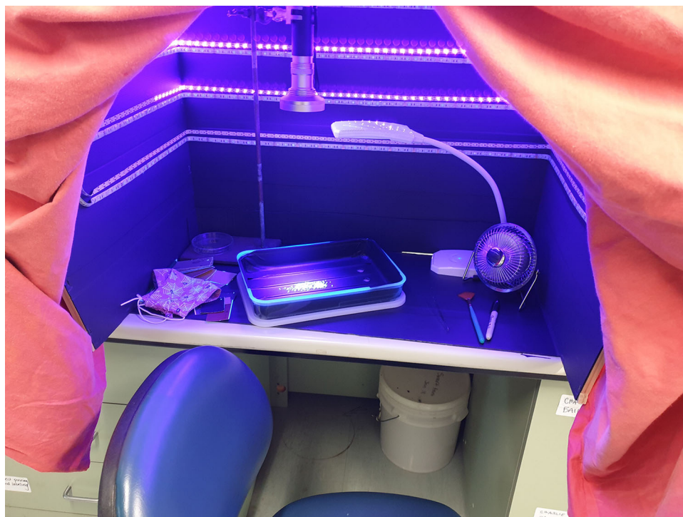
FIGURE A2 The light box used to illuminate our samples. The size of the box accommodates the observer and provides enough space to sit upright comfortably and maneuver freely to sort the pellet samples (box measured 75 cm deep at the top [60 cm at the bottom] \times 60 cm tall \times 60 cm wide). In this photo, the HEVL LED light strips are illuminated, as is the HEVL flashlight held in the clamp of the retort stand. Visible on the right is the visible light lamp with adjustable flexible arm used to illuminate the sample in conjunction with the visible light LED strip lights. The low-speed fan pictured was used to cool the observer inside the box. The observer wore eye protection to shield their eyes from HEVL light.
