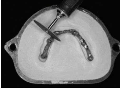
FIGURE 3: Splitting of the framework with a carborundum disc.
