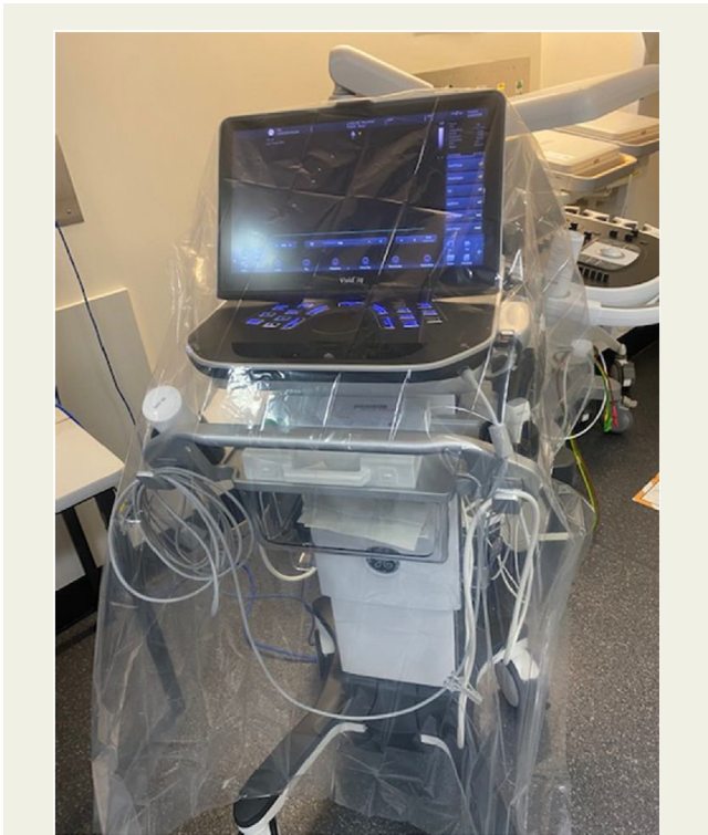
Fig. 1 When scanning COVID-19 patients, the ultrasound machine can be covered using the plastic drapes.
