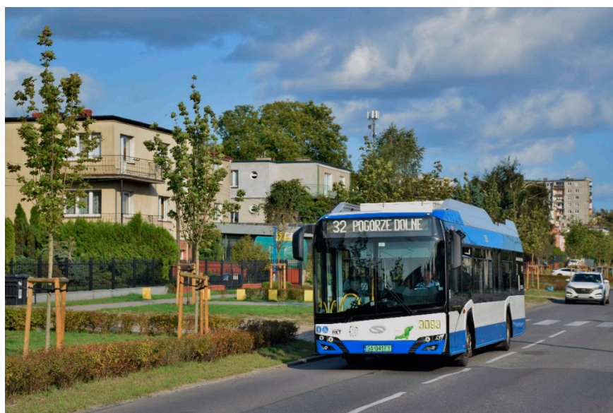
Figure 3. A trolleybus running on line 32 using battery power in Gdynia (photo taken by M. Połom).
