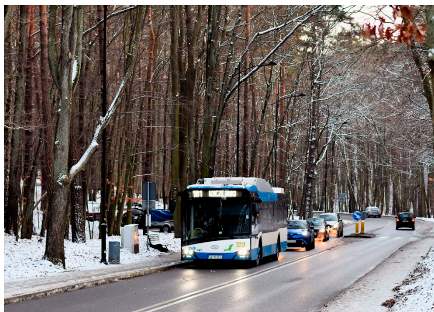
Figure 4. A trolleybus running on bus line 181 using battery power in Sopot (photo taken by K. Grzonka).
