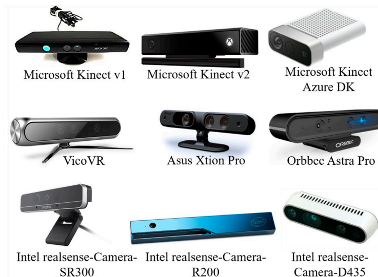
Figure A1. Recent RGB-D sensors: structured-light (Kinect v1, Asus Xtion Pro, Intel SR300), time-of-flight (Kinect v2, Kinect Azure DK, VicoVR), and active stereo vision (Intel R200, D435).
