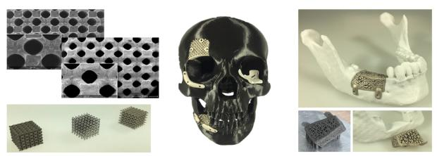
Figure 12: 3D printing of magnesium implants using selective-laser-melting (SLM)
