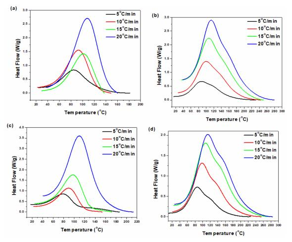
**Figure 1.** DSC thermographs of the (**a**) neat epoxy, (**b**) epoxy/P-HNT, (**c**) epoxy/A-HNT and (**d**) epoxy/F-HNT at four different heating rates of 5, 10, 15 and 20 °C min<sup>-1</sup> [27].
