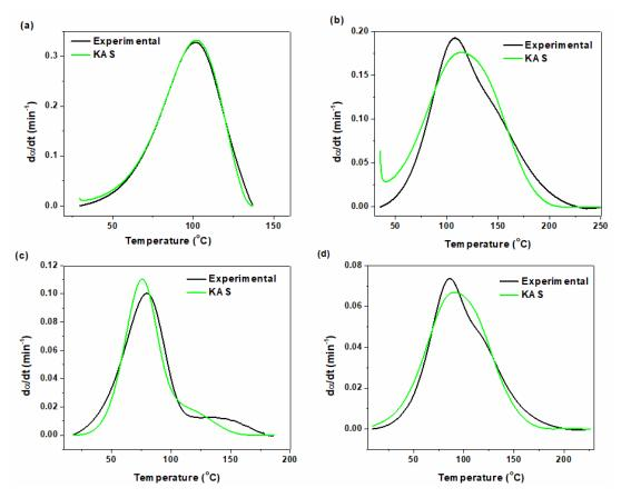
**Figure 13.** Comparison of experimental data with the kinetic models for (**a**) neat epoxy, (**b**) epoxy/P-HNT, (**c**) epoxy/ A-HNT and (**d**) epoxy/ F-HNT based on *KAS* model.
