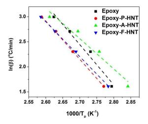
**Figure 8.** Plots of  $ln(\beta_i)$  vs. 1/T for neat epoxy, epoxy/P-HNT, epoxy/A-HNT and epoxy/F-HNT nanocomposites based on *FWO* model.
