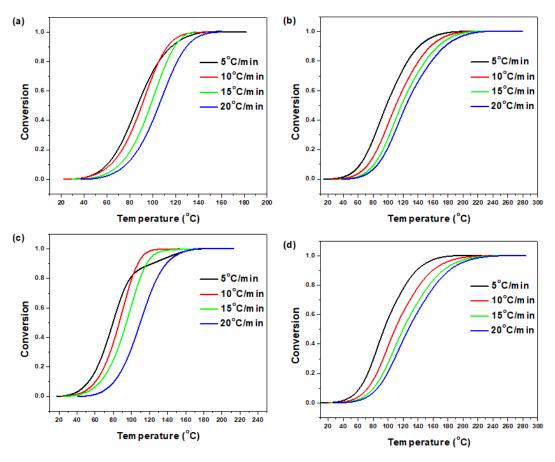
**Figure 2.** Fractional extent of conversion for neat epoxy and its nanocomposites at heating rates of (a) 5, (b) 10, (c) 15 and (d) 20 °C min<sup>-1</sup>.
