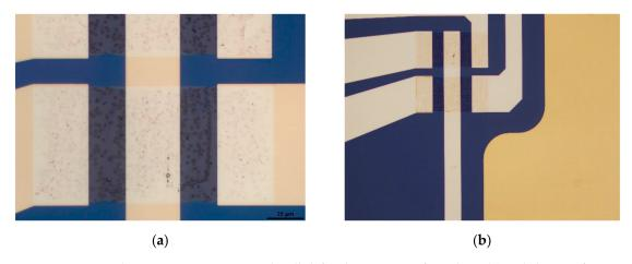
Figure 8. Optical microscope images reveal well-defined patterning of graphene (a) and clean surfaces after removing the sacrificial layer (b).
