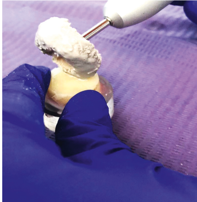
FIGURE 4: Polishing of polymethylmethacrylate blocks.
