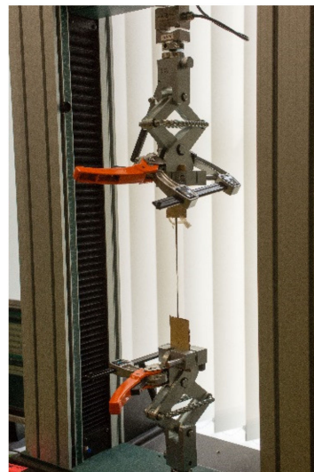
Figure 4. Set-up for the basalt fiber anchorage length and tensile strength measurements.
