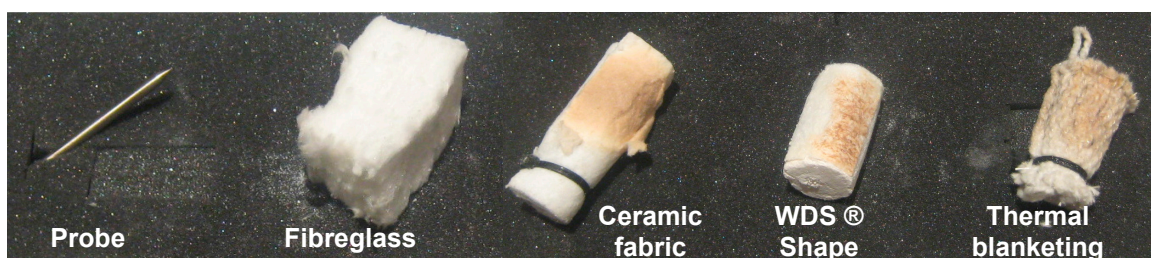
Figure 5. Insulating materials tested: ceramic fabric, WDS ® Shape, thermal blanketing, and fibreglass.
