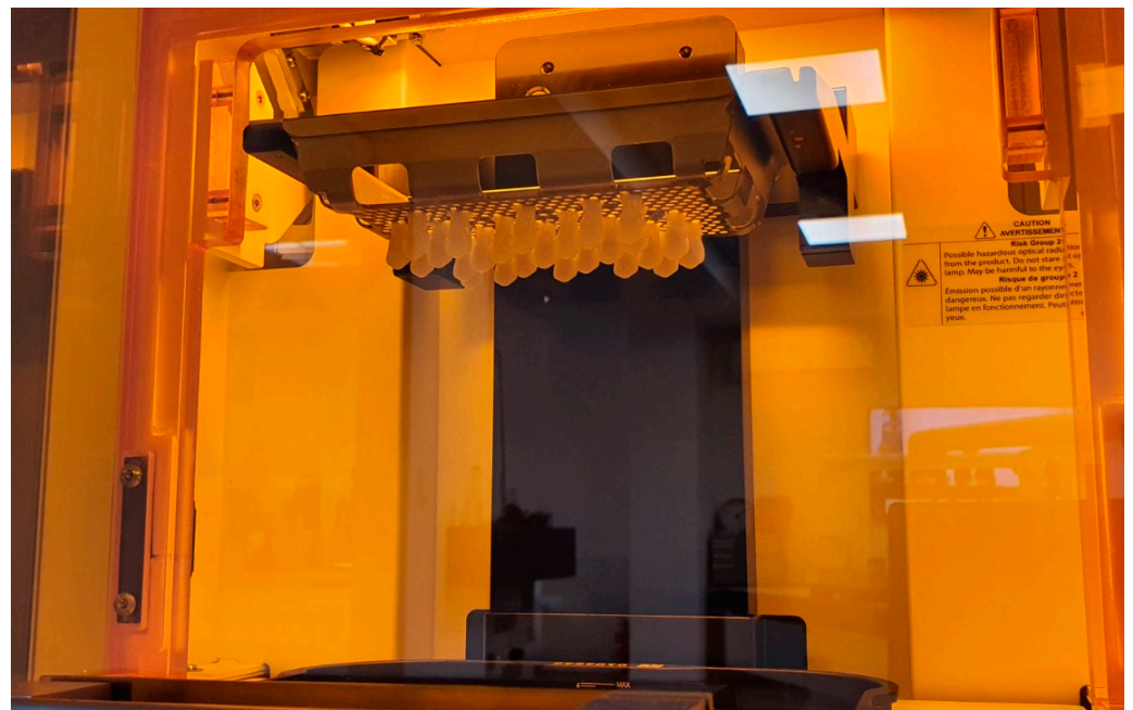
Figure 2. Three-dimensional printing of the artificial teeth: dental resin material NextDent C&B MFH (NextDent 3D Systems, Soesterberg, The Netherlands) is placed into the 3D printer NextDent 5100 (NextDent, 3D Systems, Soesterberg, The Netherlands).
