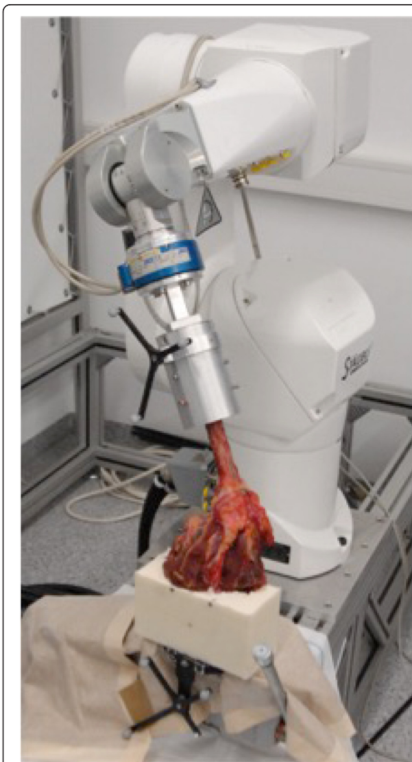
Fig. 2 Shoulder specimen with the robotic testing system. Legend Table 1: T1: knot technique, T2: pulley technique, T3: tape technique, I: Intact native specimens. Legend Table 2: T1: knot technique, T2: pulley technique, T3: knotless suture tape technique (T3 vs. T1/T2 p = .03 ; T1 vs. T2 n.s.)
