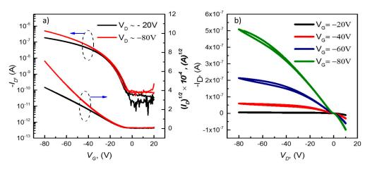
**Figure 4.** Representation of (**a**) transfer curve (**b**) output curve of PTPABDT based OFETs at the optimum annealing temperature.
