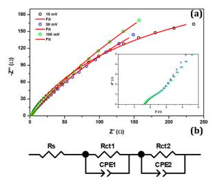
**Figure 6.** Electrochemical impedance spectroscopy (EIS) (**a**) Nyquist plots of triphenylamine based hyperbranched polymer with various applied bias potential and (**b**) Equivalent circuit model used for fitting.
