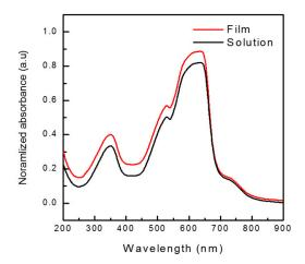
**Figure 2.** UV-vis absorption spectra of PTPABDT polymer both in solution (5 mg/mL) and in solid film state.
