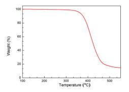
**Figure 1.** TGA plots for the polymer, obtained with a heating rate of 10  $^{\circ}$ C min<sup>-1</sup> under an inert atmosphere.
