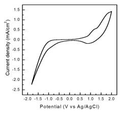
**Figure 3.** Cyclic voltammograms of PTPABDT in 0.1 M  $Bu_4NPF_6/CH_3CN$ , scan rate 50 mV s<sup>-1</sup>, Pt working electrode.
