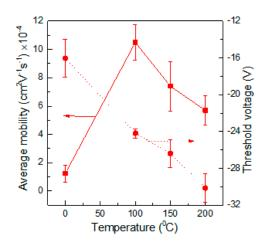
**Figure 5.** Graphical representation of the trend of average field-effect mobility and threshold voltage dependence on annealing temperature of the PTPABDT film.
