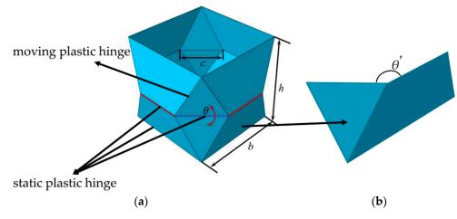
**Figure A2.** (a) A module of OCB; (b)  $\theta'$ .
