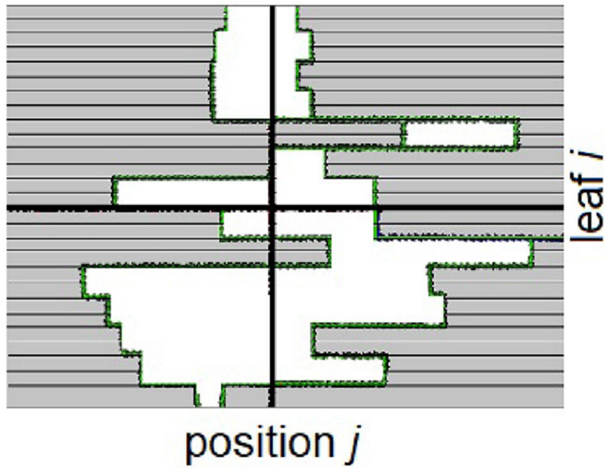
Fig. 3. An example of an aperture (white, unshaded) formed by collimator leaves.
