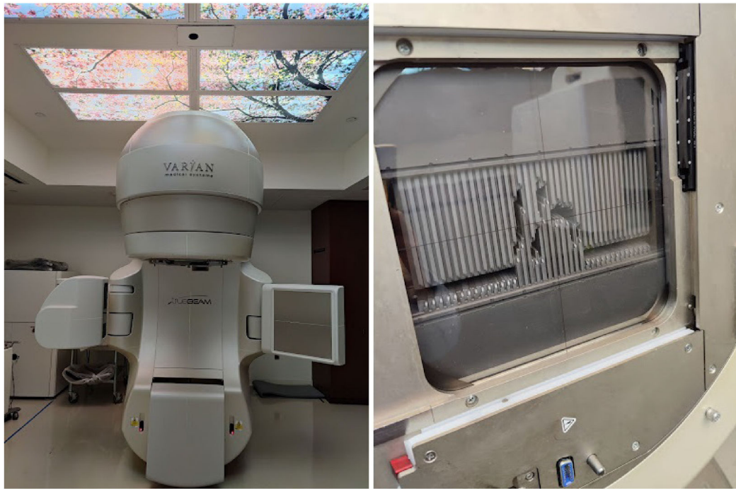
Fig. 1. (Left) Varian TrueBeam LINAC and (right) its MLC comprised of tungsten leaves to shape the radiation beam delivered by the LINAC.
