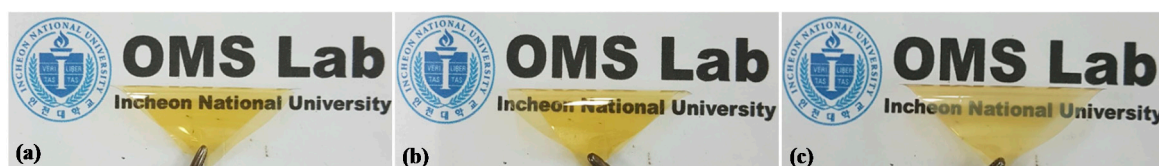
Figure 3. Pictures of the [(PIM-PI) x -(6FDA-durene-PI) y ] copolymer membranes with 1:4 (a), 1:6 (b) and 1:10 (c) compositions.
